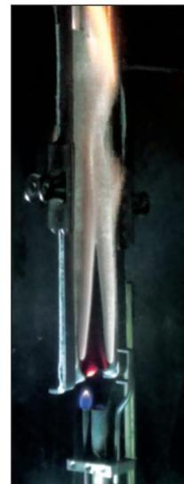
Vertical flame test on generic FR fabric — significant after flame
