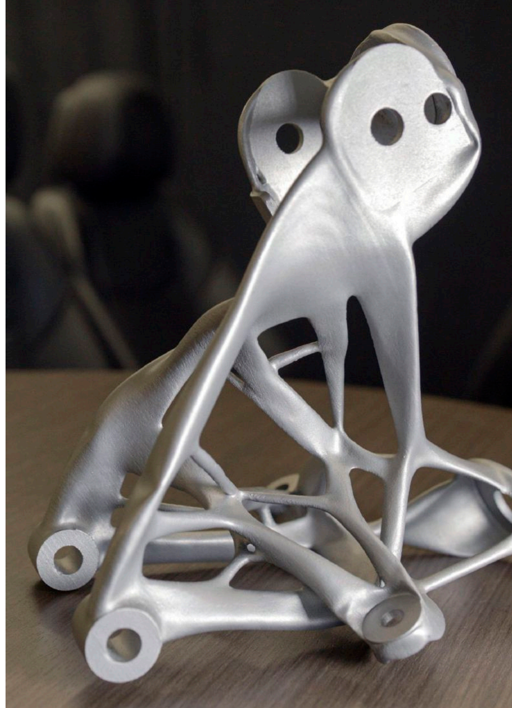
GM consolidated an eight-part seat bracket into a single part using generative design and additive manufacturing. Courtesy of General Motors.
