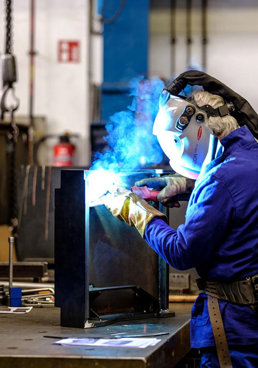
A welder fabricates the prototype for the new transport part, reverse-engineered using ideas from generative design, traditional design, and input from the foundry. Courtesy of Claudius Peters.
