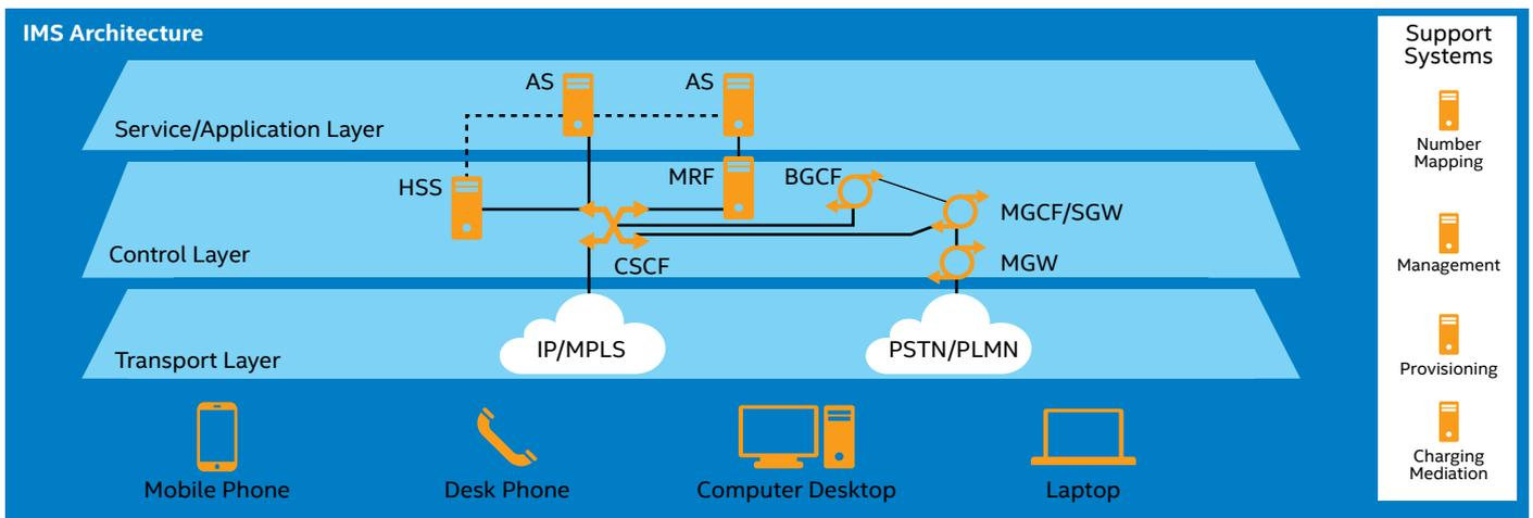
Figure 2. IMS contains layers and elements that can be abstracted from the underlying hardware through virtualization
